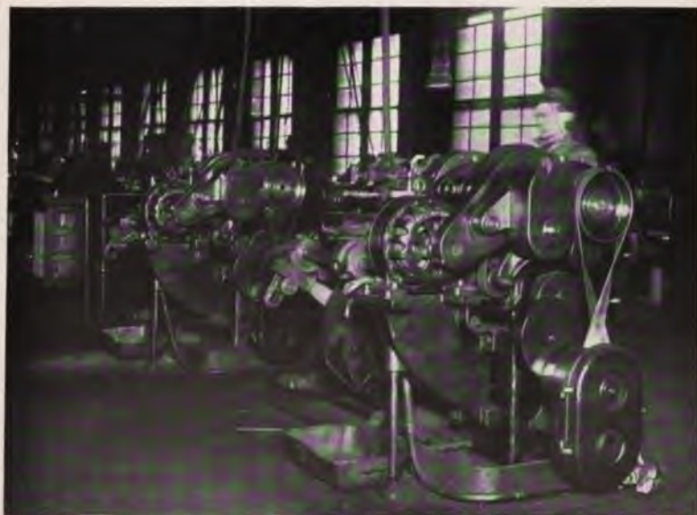
TURRET LATHES, ALL GEARS GUARDED
